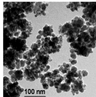
**Figure 1.** TEM photograph of the as-prepared amorphous Ni–B alloy.
